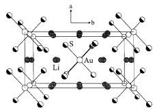
Figure 2. Unit cell of Li<sub>3</sub>AuS<sub>2</sub> along [001] showing the Au····Au interactions.
